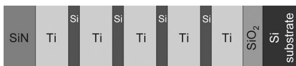
Fig. 1. Schematic structure of Ti/Si multilayer system created on Si-substrate and capped with SiN layer.
